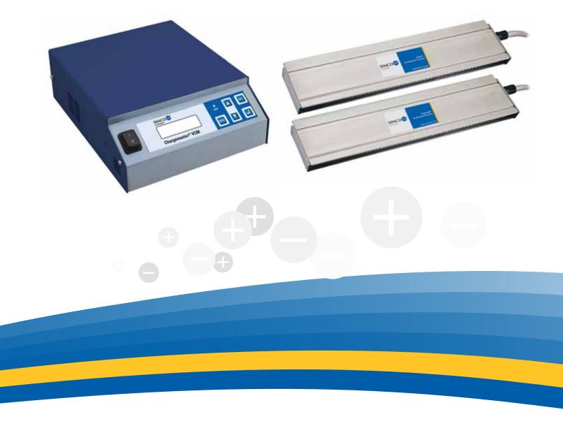
Chargemaster systems utilize high frequency switching technology, which offers three major advantages. First, it ensures that the voltage output from the power supply is equal to the voltage requested via the controls. Second, fluctuations on the AC input line will not affect the voltage output. Finally, variances in load, up to the recommended maximum, do not affect the voltage output.
